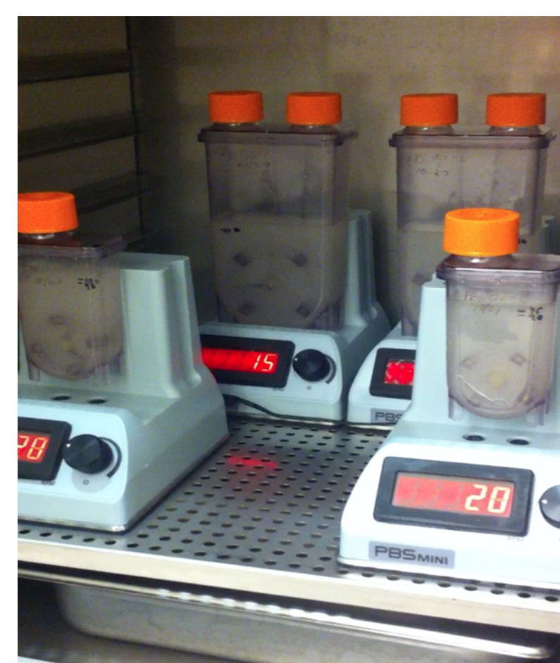
Fig 4. PBS-MINI units in operation inside a humidified CO 2 incubator. PBS-0.1 units are in the foreground and PBS-0.5 are in the back.
