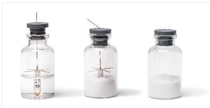
Figure 4: Tempris Wireless Sensor for Product Temperature Measurement
