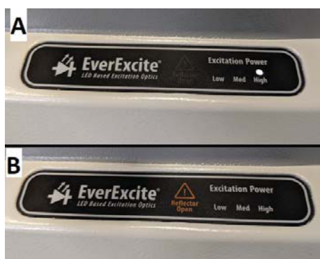
Figure 2. (A) Excitation on High (B) Reflector Open
