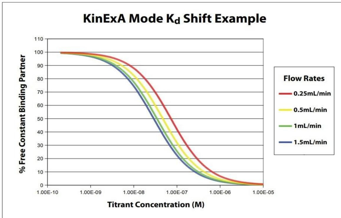
Figure 1. The best  $K_d$  is 2.2 times tighter at 1.5 mL/min when compared to 0.25 mL/min.
