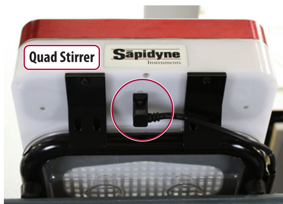
Figure 4. Serial cable connection to the Quad Stirrer.
