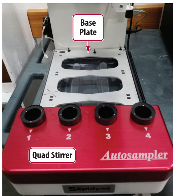
Figure 3. Installation of the Base Plate with the Quad Stirrer.
