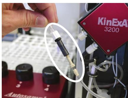
Figure 2. Connecting the Autosampler and KinExA Buffer Lines.
