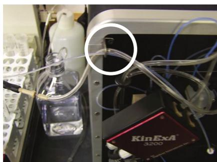
Figure 6. Sample Line routed through the Tubing Support.
