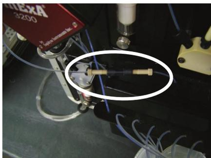
Figure 5. Connecting the Flow Cell and the Autosampler Sample Line.
