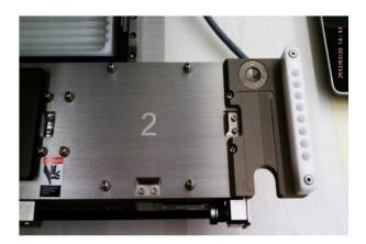
The LCP Arm is a syringe drive that allows low volume fluid handling independent of high viscosity solutions typical of protein seed stock stabilization mixtures.
