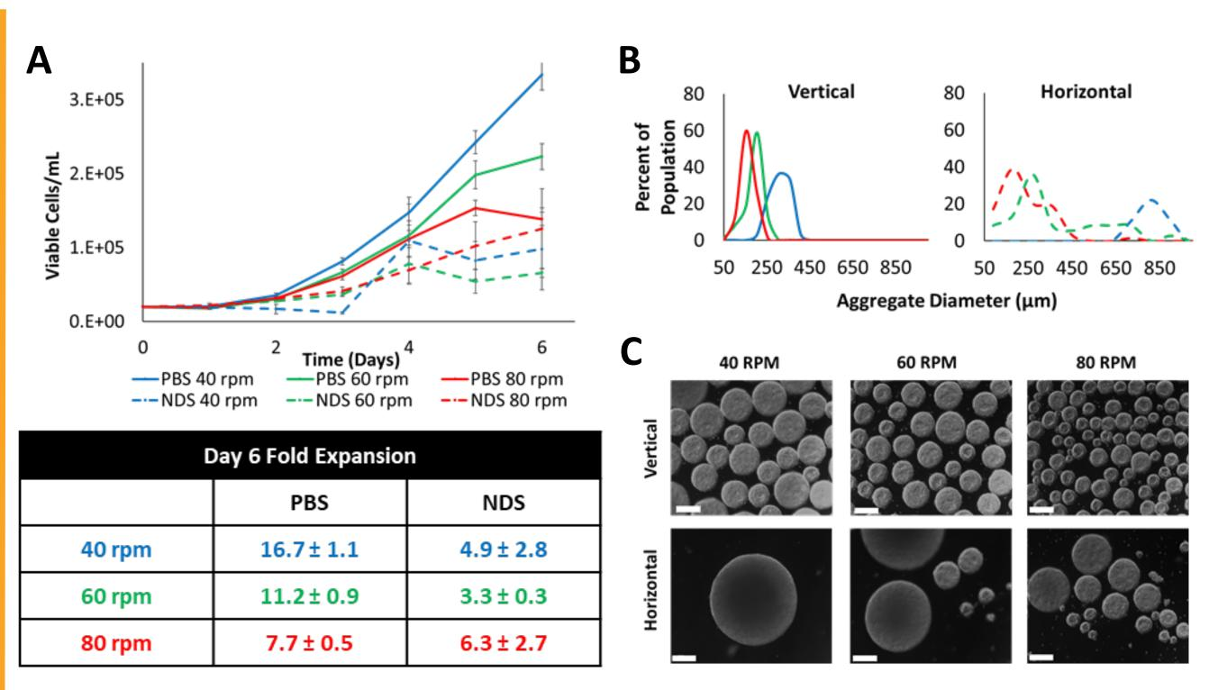
Figure 1: Single cell expansion was successful in VW bioreactors, but not in traditional horizontal-blade bioreactors as demonstrated by the growth kinetics (A). The VW bioreactor also resulted in more uniform aggregate size distributions as shown in the Day 6 distributions (B) and images (C). Scale represents 200  $\mu$ m.
