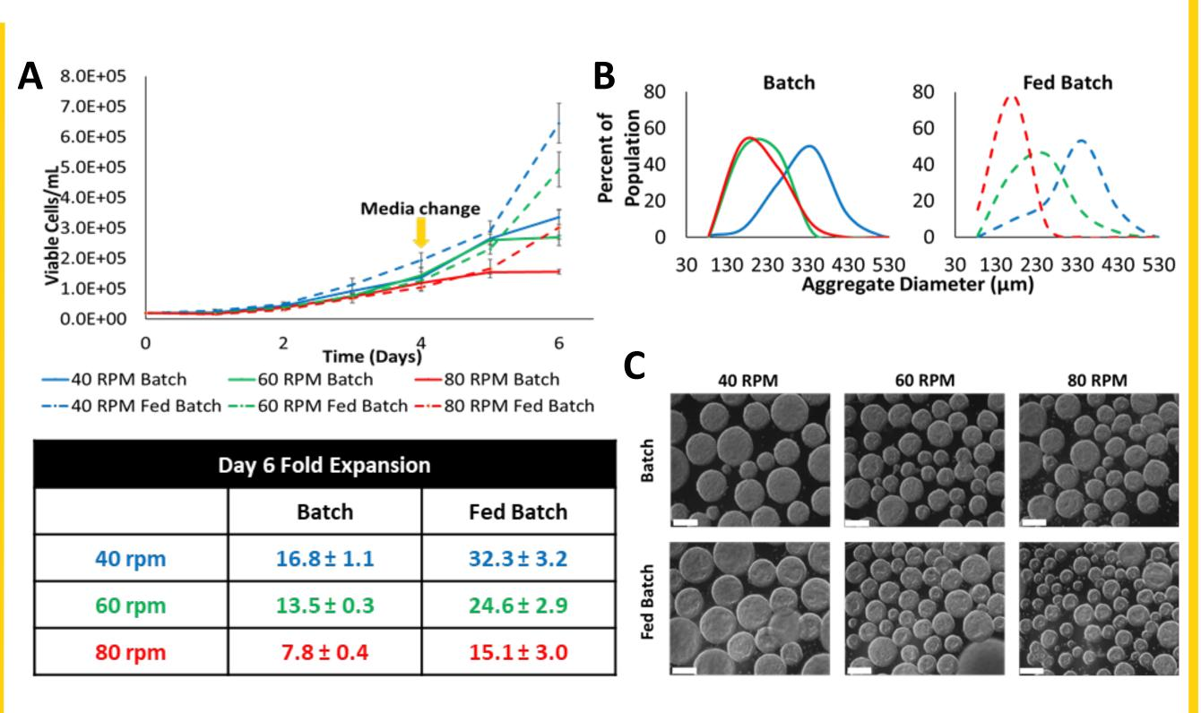
**Figure 2:** Fed-batch culture in VW bioreactors resulted in approximately 2 times higher cell expansion at all agitation rates with a maximum of 32 at 40 RPM **(A)**. The use of a fed batch strategy also resulted in more optimal aggregate diameters as shown in aggregate size distributions **(B)** and pictures from Day 6 **(C)**.
