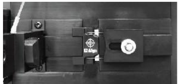
Figure 1. Orientation of the EZ Align Tool installed in the Flow Cell Groove.
