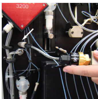
Figure 4. Pulling the connector through the hole.
