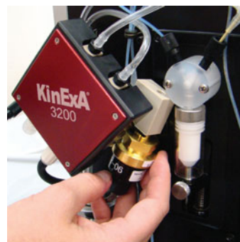
Figure 3. Removing the pressure transducer from the mount.
