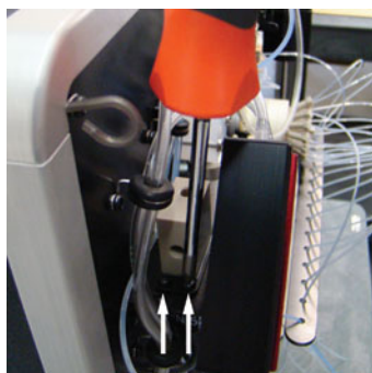
Figure 2. Removing the screws located to the left of the pressure transducer.
