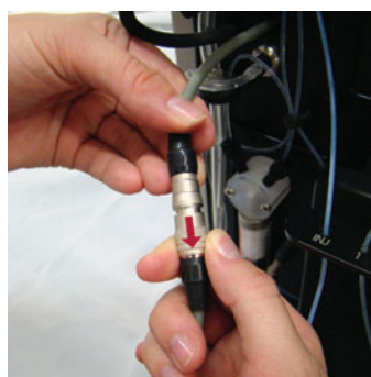
Figure 5. Disconnect the connector by pulling the top part away from the instrument.
