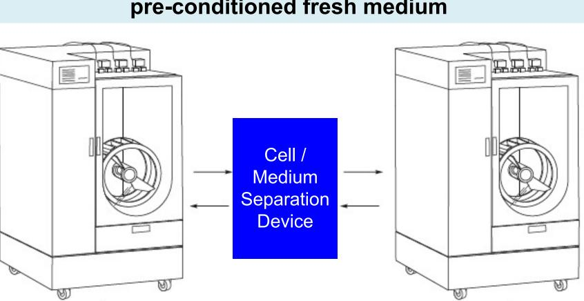
Figure 10. A methodology for using an external separation and retention device in conjunction with multiple bioreactors to facilitate rapid, scalable medium exchange
