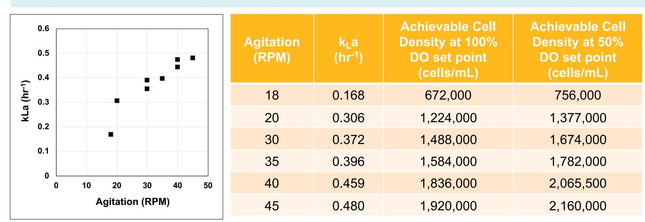
**Experimental Condition Assumptions:**  Vessel: PBS-3 MAG bioreactor Specific oxygen consumption rate,
