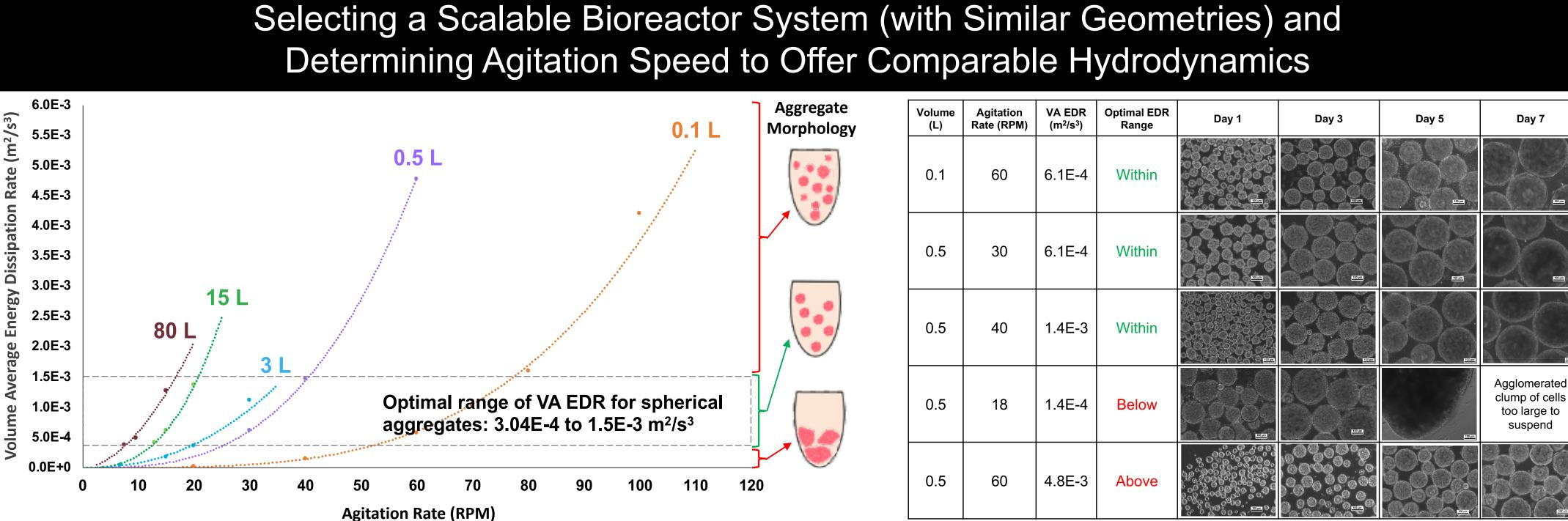
Figure 5. Curves to determine volume average (VA) energy dissipation rate (EDR) based on VW bioreactor working volume and agitation rate. Average EDR can be used to predict aggregate morphology for a particular combination of volume and agitation, with desired spherical aggregates, a consequence of average EDR within an optimal range.
