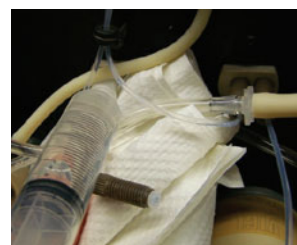
Figure 5. Pushing dH 2 O through the solenoid valve.
