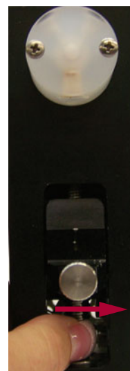
Figure 2. Twist the lead screw to the right to lower the syringe platform.
