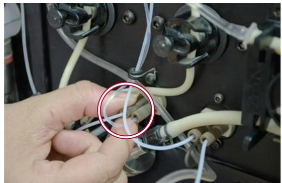
**Figure 2.** Disconnect the nut from the left side of the solenoid valve on the left.
