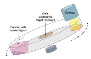
over the elevated part of the dish, measures the signal intensity from both the cell area and a reference area (cell free or another cell line), which enables a continuous subtraction of the background signal from the cell line of interest every revolution. As the ligand interacts with the cells over time, an increasing or declining response is generated, representing the association and dissociation rates of the interaction.
