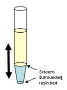
This is the typical PhyNexus PhyTip column format, showing the media (or resin) lodged at the bottom of the tip between filter screens, providing a way to aspirate and dispense reagents over the media bed volume using a pipette action. The Scorpion's ability to move slowly and precisely is useful for this technology.
