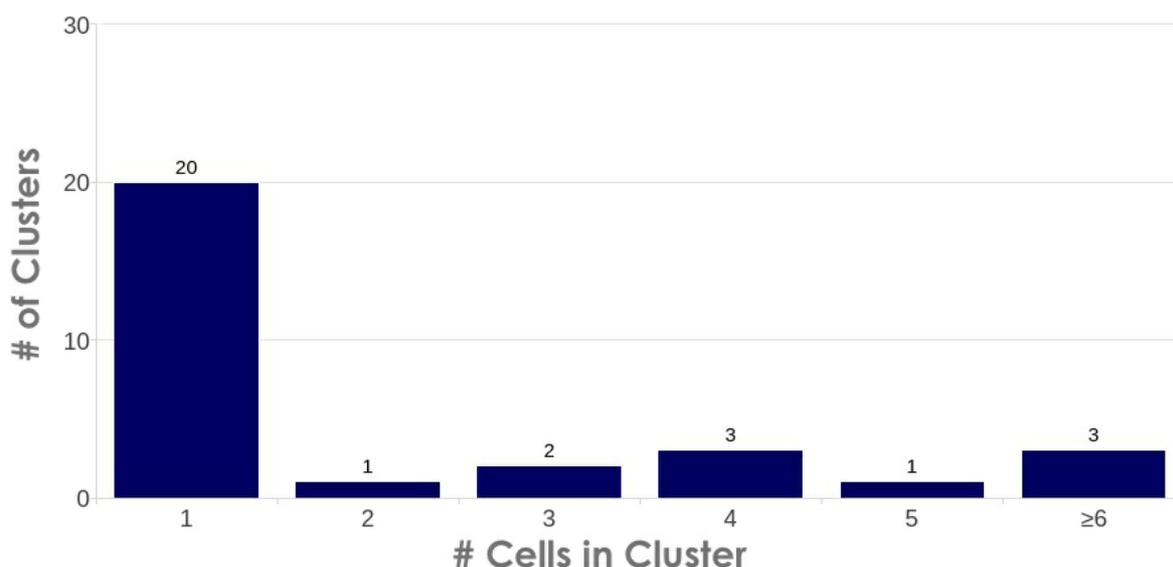
Figure 2: Count cluster data from the CellDrop. When CellDrop counts cells/nuclei it also analyzes the result for clusters of objects. The software allows the user to visualize the cluster size and the frequency of up to six different cluster sizes for each count on the device.
