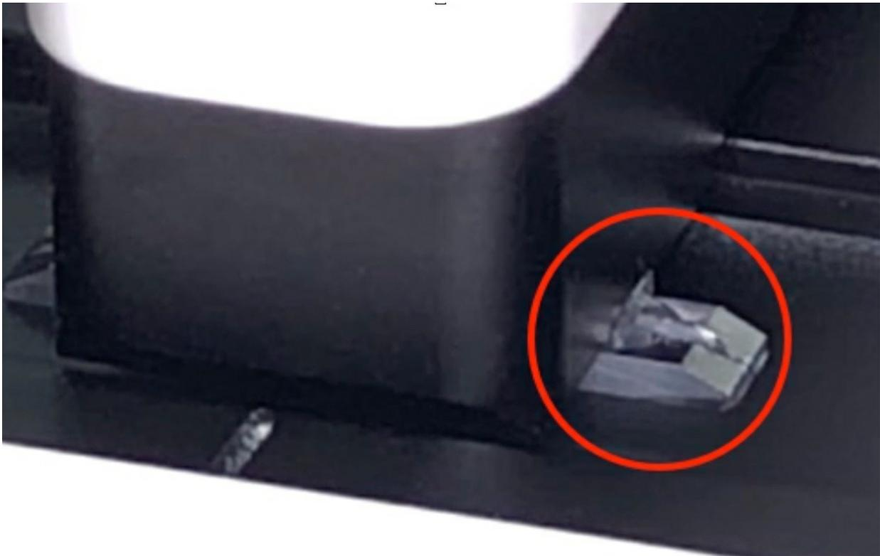
Figure 4: Sample not loading. Static charge prevents capillary action of the liquid sample
