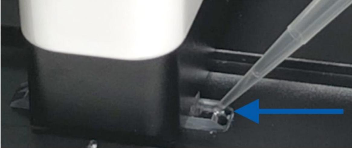
Figure 2: Pipette position for cleaning. Load 70% ethanol into the alignment groove.
