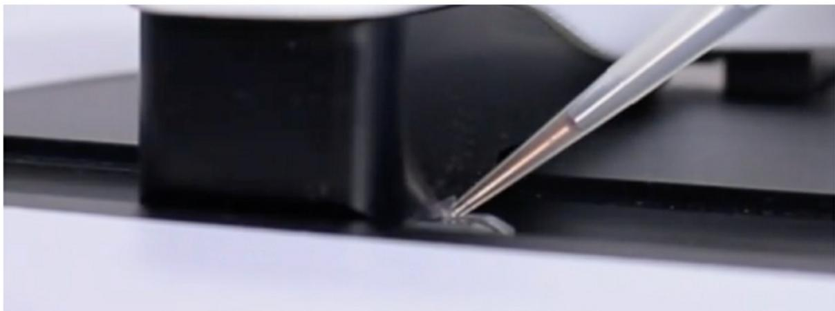
Figure 1: Loading. Rest pipette tip against upper surface while dispensing sample.
